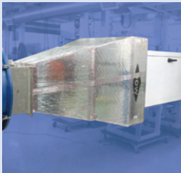
Airflow tests measure output and validate actual heat dissipation
