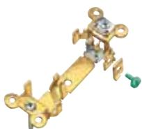
One piece, all brass, mounting strap with integral ground contacts. The safest, most reliable design for a low resistance flow of fault currents. Oversized "bell" shaped ground contacts, along with nickel plated steel retaining shields, help minimize damage to the grounding system during abrupt pullout. Barbed brass locking arms keep the face locked in place to diminish potential for face/base separation. Back wired ground terminal reduces installation time and increases convenience.
