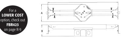
Mounts easily and securely between joists...adjusts from 16" to 24" o.c.
