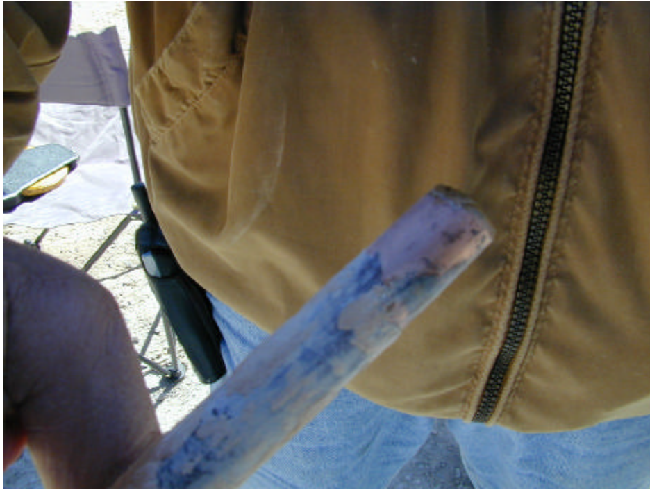
Figure 3. Close-up of 5/8" x 8' copperbonded rod after 10 years. Electrode type H.
