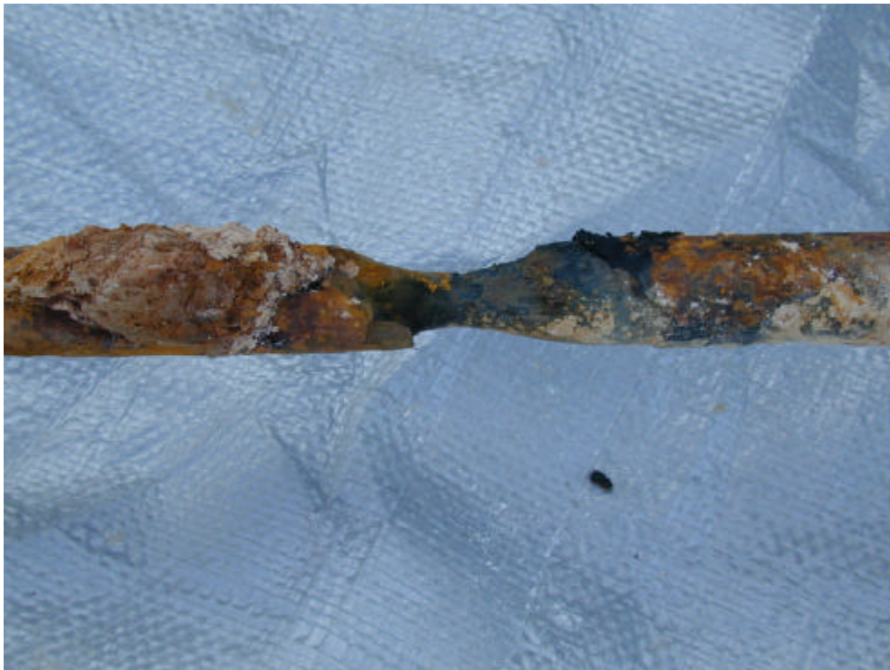
Figure 4. Close-up of 3/4" x 10' galvanized rod after 10 years. Electrode type I.
