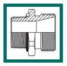
These Tuff-Seal RSR grips feature an O-ring that creates a watertight seal when they are used in a taper tapped conduit hub. In these applications gaskets must be used in either the knockouts or clearance drilled holes. To ensure a more reliable seal an embedded O-ring should be utilized. Many of the standard Tuff-Seal cord grips listed
