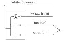
As an Input to a BZ-150 Power Pack for Manual-on Operation
