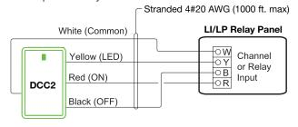
As shown at the left, the DCC2 LED is a Pilot Light. To use the LED as a locator, connect the yellow wire to the panel's 24V supply.
